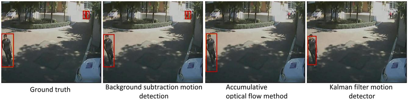
Figure 4: Examples of the motion detection results on a sample frame. First image represents the ground truth (three moving objects), the second image shows results of the background subtraction motion, the third present the performance of accumulative optical flow method, and the fourth image present an example for Kalman filter motion detector.
