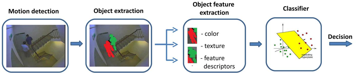
Figure 1: The proposed automated surveillance system.
